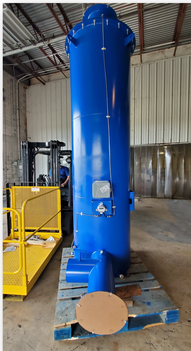
Single Fiber Bed Filter Vessel
