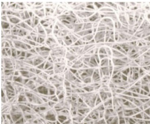
Close-up image of typical knitted mesh media
