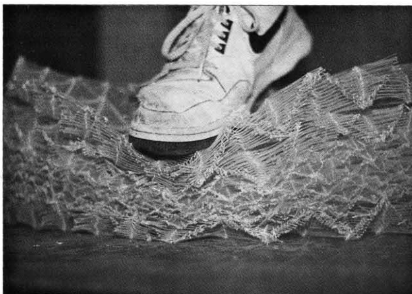
Provided sustained pressure is avoided, Kimre pads do not require especially careful handling; they can withstand fairly robust treatment in transport and installation.
